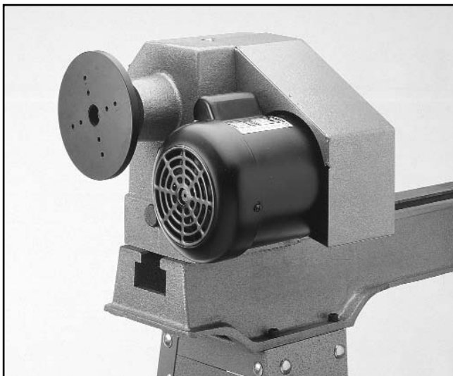
Figure 22. Headstock set at 180°.
